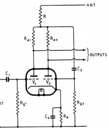
Fig. 3. Common-anode-coupled phase splitter. Typical values:  $V_1$ ,  $V_2$ , = 6SN7,  $R_{\sigma 1} = R_{\sigma 2} = 1M\Omega$ ,  $R_k = 1.8 k\Omega$ ,  $R = 39 k\Omega$ ,  $R_{a1} = 80k\Omega$ ,  $R_{a2} = 100 k\Omega$ ,  $C_1 = 0.05 \mu F$ ,  $C_2 = 0.25 \mu F$ ,  $C_k = 20-50 \mu F$ , h.t. = 350V. Gain (input to one output) = 17 (approx.).
