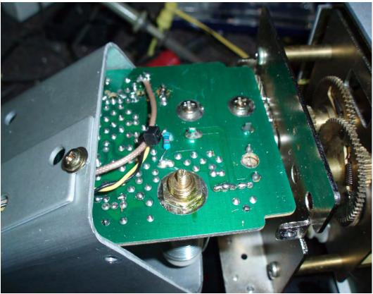
VFO Can Removed, 10k Resistor and 2 Connections
