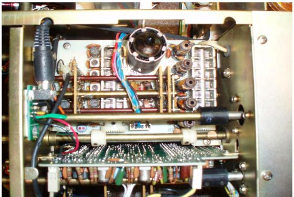
Driver Board with DD-103 Interface View
