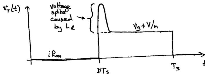
If the peak magnitude of the voltage spike exceeds the voltage rating of the MOSFET, then  $Q_1$  will fail.
