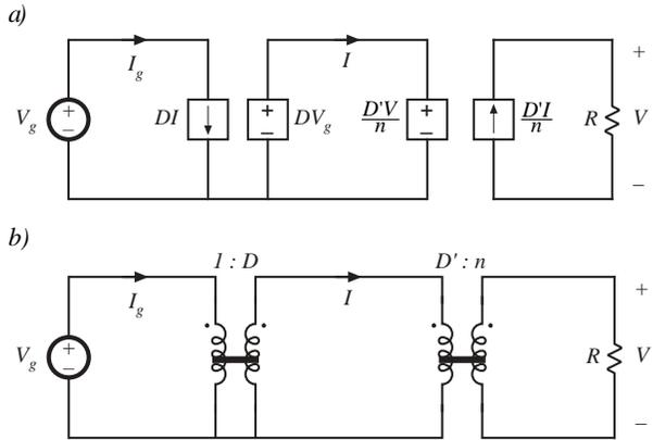
Fig. 4. Flyback converter equivalent circuit model: (a) circuits corresponding to Eqs. (5), (7), and (9); (b) equivalent circuit containing ideal dc transformers.
