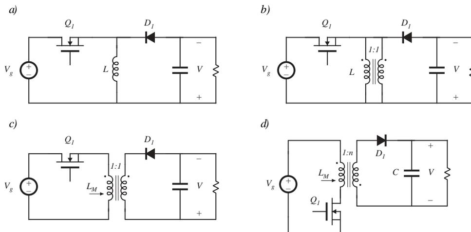
Fig. 1. Derivation of the flyback converter: (a) buck-boost converter, (b) inductor  $L$  is wound with two parallel wires, (c) inductor windings are isolated, leading to the flyback converter, (d) with a 1:n turns ratio and positive output.
