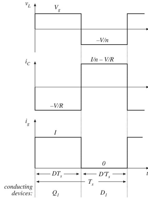
Fig. 3. Flyback converter waveforms, continuous conduction mode.
