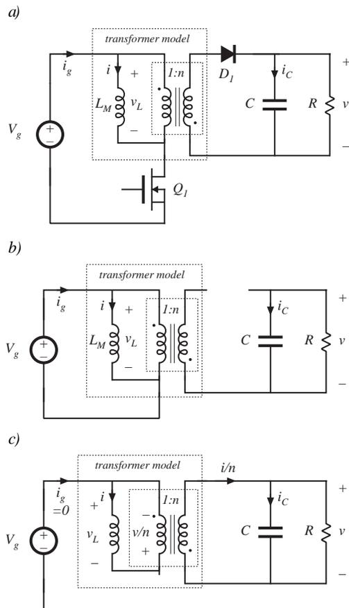
Fig. 2. Flyback converter circuit, (a) with transformer equivalent circuit model, (b) during subinterval 1, (c) during subinterval 2.
