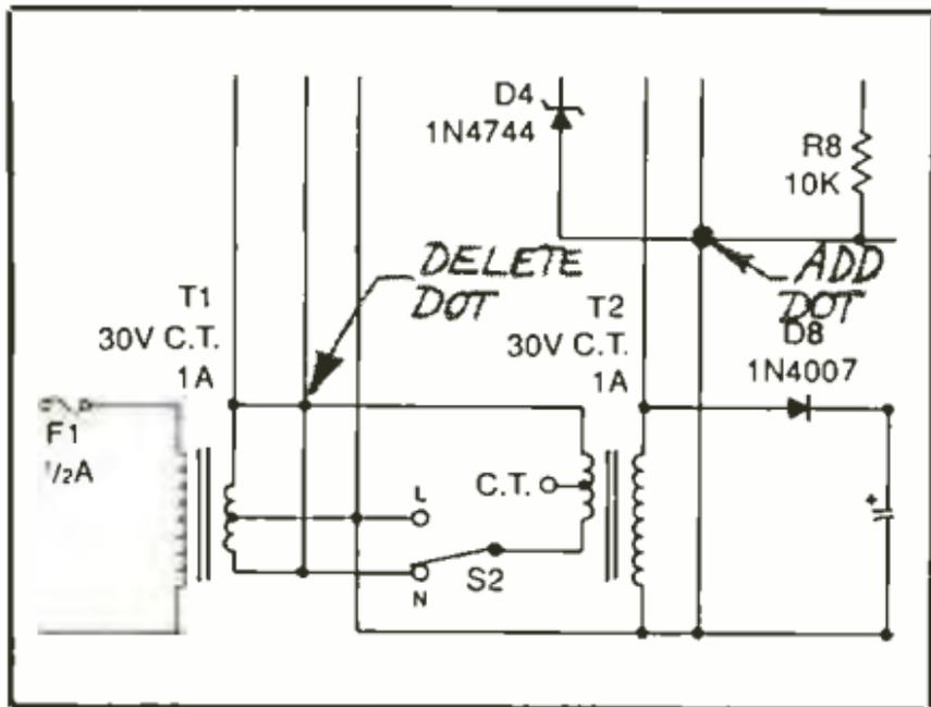
*The "Telephone Tester" schematic is in error. Schematic corrections are shown here.—Ed.*
