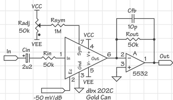
Figure 3. dbx 202C with internal current correction circuitry
