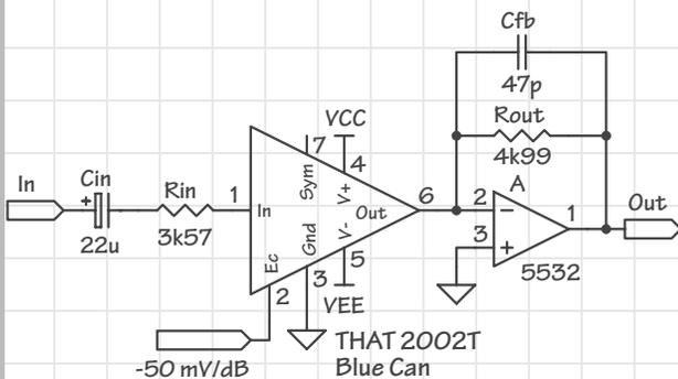
Figure 12. The recommended schematic for the THAT 2002T
