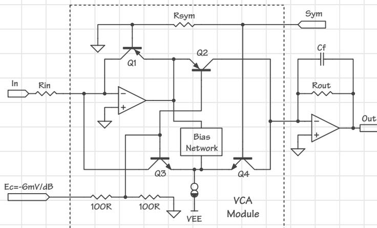
Figure 1. Simplified schematic of a log/anti-log VCA
