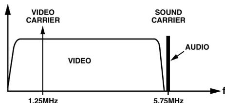
The frequency information may be misleading to a reader not familiar to the standard. More commonly, the audio carrier frequency is measured relative to the channel carrier frequency or the video carrier frequency. The audio subcarrier would be 4.5 MHz. It is more intuitive to view the spectrum as seen below:
