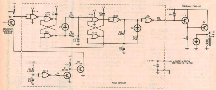
The following is a description of the additions which I have made to the 10GHz Radar Burglar Alarm, described in July, 1977. It provides exit and entry delays
