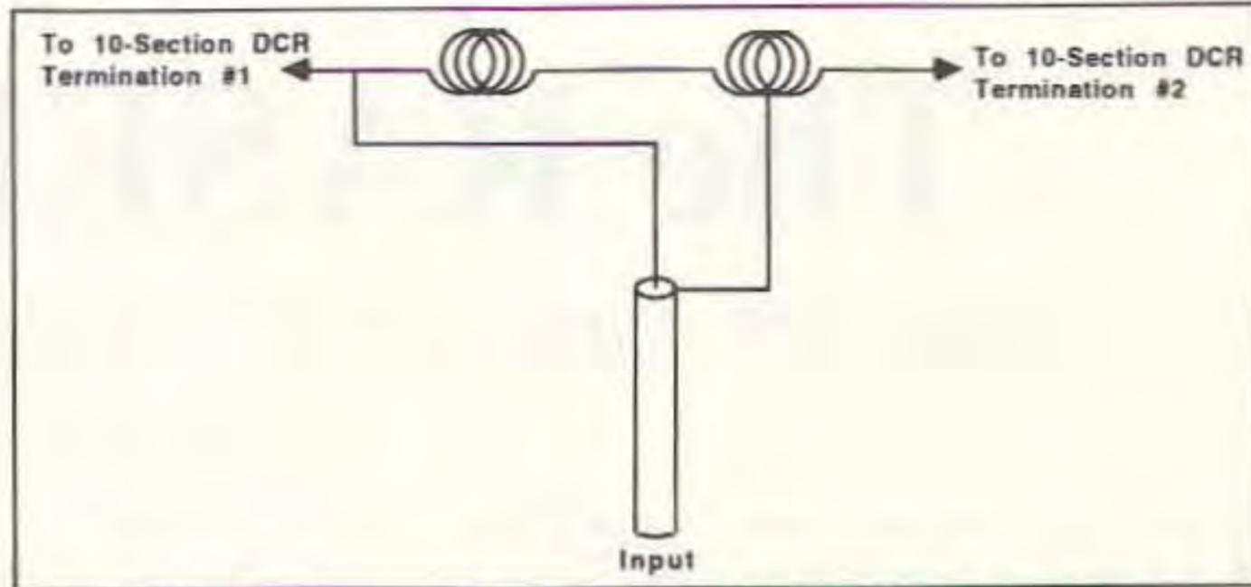
Figure 6. Improved balanced coupler unit (no capacitor).
