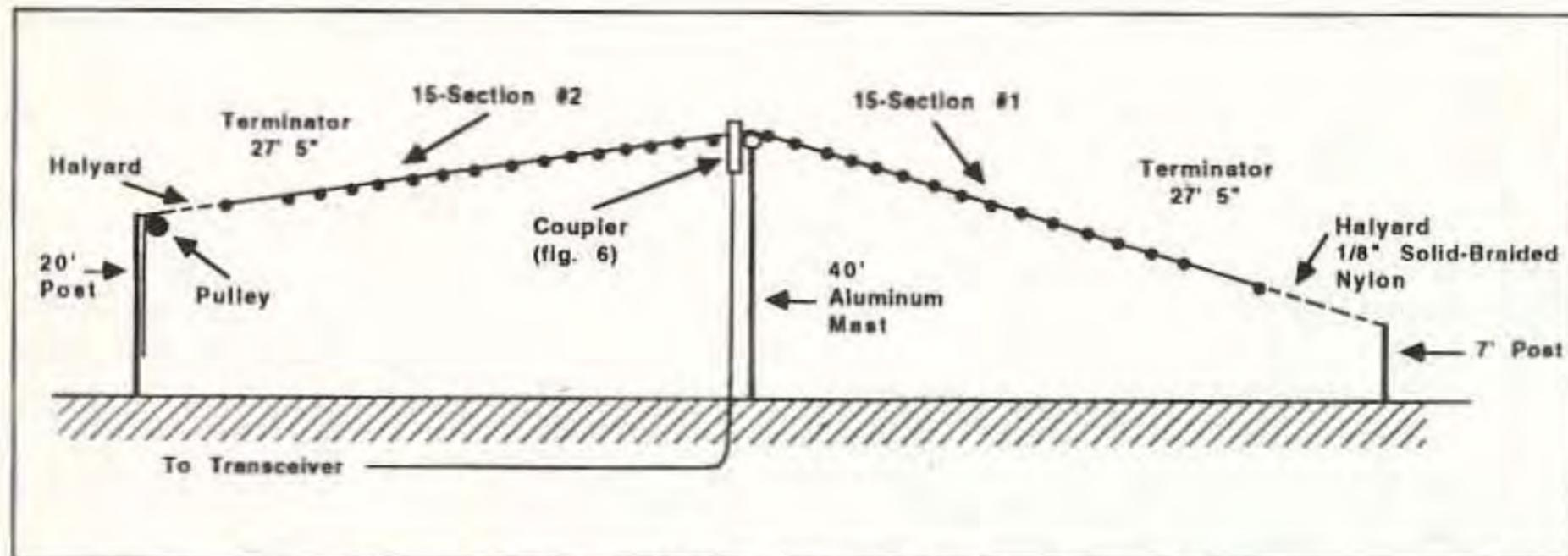
Figure 7. Balanced 30-section RASER—(center-fed).
