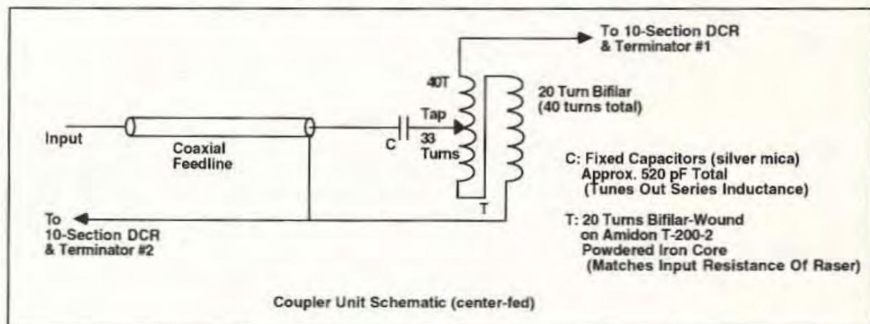
Figure 3. Coupler unit schematic (center-fed).
