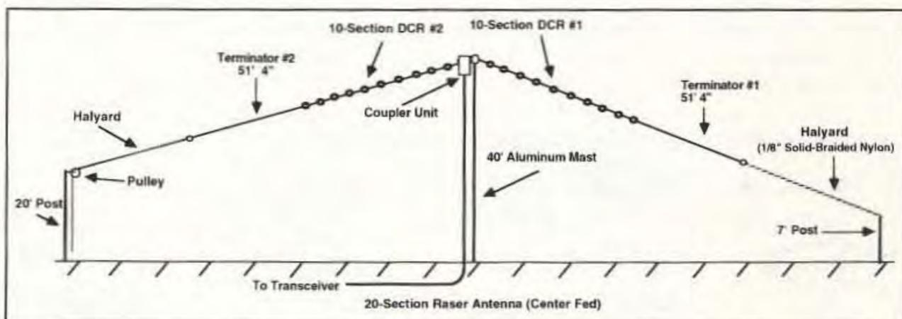
Figure 1. 20-section RASER antenna (center-fed).
