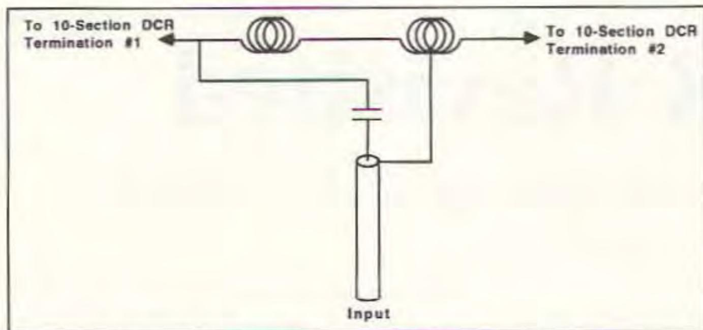
Figure 5. Original coupler unit—balanced input.
