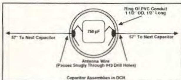
Figure 2. Capacitor assemblies in the DCR.
