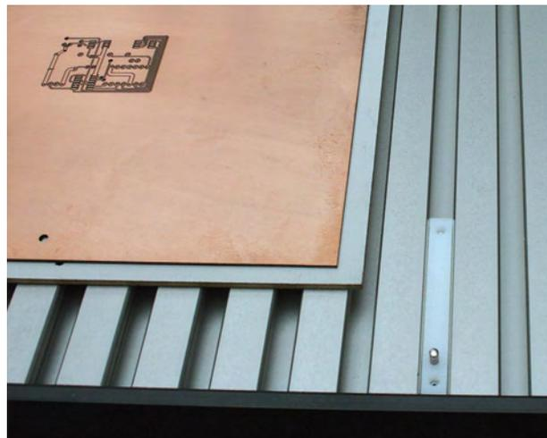
or bowed (within certain limits, of course) – the milled channels will always have a constant width. As floating cutter heads are usually adapted to the spindle motor that is used, they are difficult to find as commercial products. However, it's fairly easy to make one yourself once you understand the principle.
