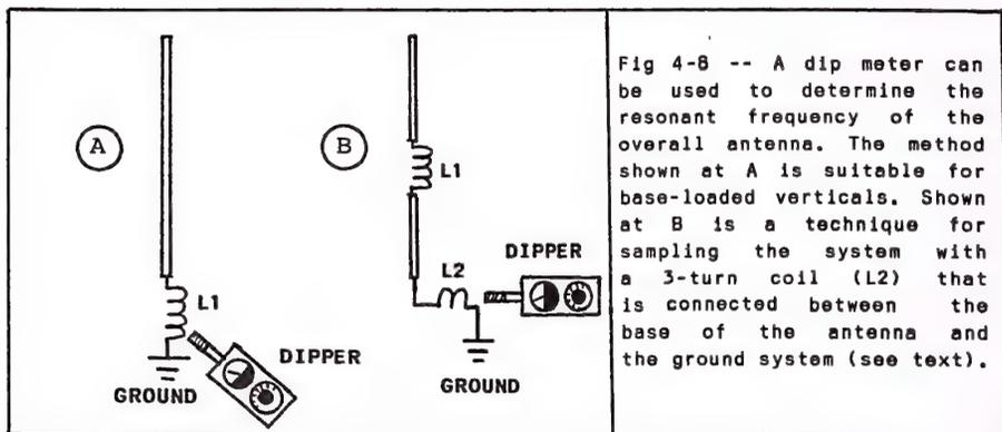
Fig 4-8 -- A dip meter can be used to determine the resonant frequency of the overall antenna. The method shown at A is suitable for base-loaded verticals. Shown at B is a technique for sampling the system with a 3-turn coil (L2) that is connected between the base of the antenna and the ground system (see text).
