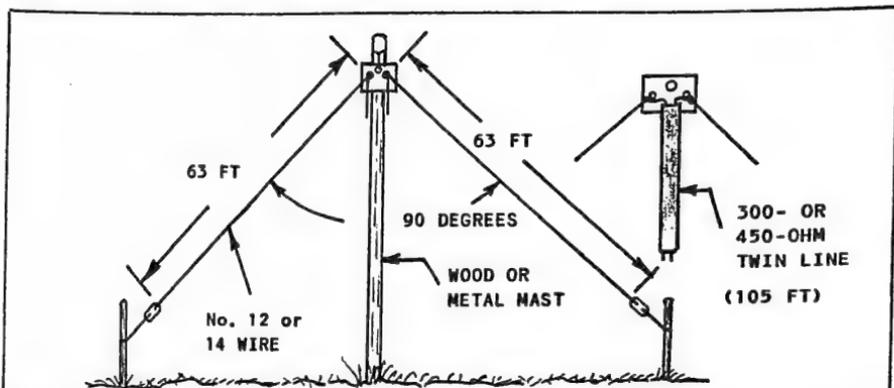
Fig 2-10 -- Multiband inverted-V dipole with tuned feeders. The dimensions provided are for resonance at 3.725 MHz. Feeder length is  $1/2$  wavelength, inclusive of the velocity factor (0.8) for TV ribbon line. The feeder may be any convenient length near 100 feet. The enclosed angle of the dipole should be between 90 and 110 degrees for best performance.
