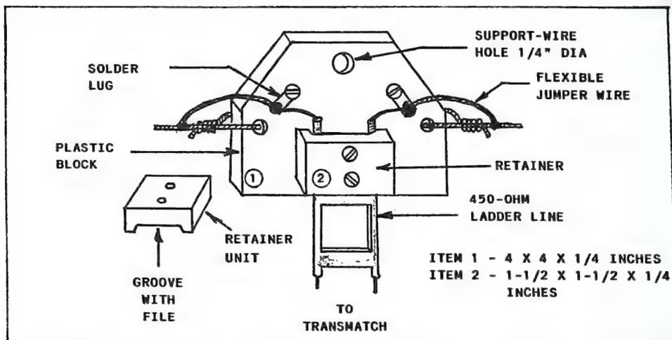
Fig 2-6 -- Example of a center insulating block for horizontal or inverted-V dipoles that are supported at the center. Other styles of feed line may be used if the retainer block (item 2) is modified to accommodate the alternative feeder, such as 300-ohm TV ribbon or coaxial cable. This homemade center insulator can be cut from sheet plastic by means of a hack saw or electric saber saw. A nylon halyard or wire support line is attached at the upper center hole of the insulator.
