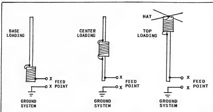
Fig 4-7 -- A short radiator may be changed to an electrical  $1/4$  wave by inserting a loading coil (inductive reactance) in series with the conductor. Base loading requires the smallest number of coil turns, while top loading has the greatest number of turns. A capacitance hat may be added to the center- and top-loaded antennas to reduce the number of coil turns.
