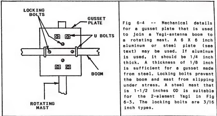
Fig 6-4 -- Mechanical details for a gusset plate that is used to join a Yagi-antenna boom to a rotating mast. A 6 X 6 inch aluminum or steel plate (see text) may be used. If aluminum is used, it should be 1/4 inch thick. A thickness of 1/8 inch is sufficient for a gusset made from steel. Locking bolts prevent the boom and mast from slipping under stress. A steel mast that is 1-1/2 inches OD is suitable for the 2-element Yagi in Fig 6-3. The locking bolts are 3/16 inch types.
