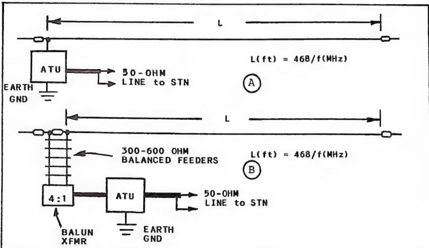
Fig 5-1 -- Two versions of half-wave, end-fed antennas. System A has the end of the wire coming directly to the antenna tuner. System B has balanced feeders from the antenna to the ham shack. Any length of feed line is satisfactory. A 4:1 balun transformer converts the balanced line to unbalanced 50-ohm coaxial cable.
