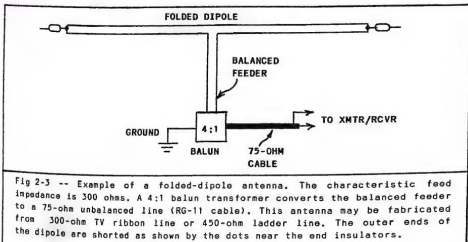
Fig 2-3 -- Example of a folded-dipole antenna. The characteristic feed impedance is 300 ohms. A 4:1 balun transformer converts the balanced feeder to a 75-ohm unbalanced line (RG-11 cable). This antenna may be fabricated from 300-ohm TV ribbon line or 450-ohm ladder line. The outer ends of the dipole are shorted as shown by the dots near the end insulators.
