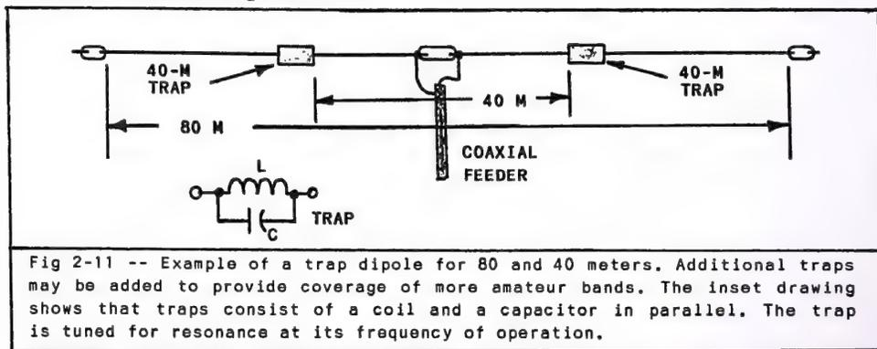
Fig 2-11 -- Example of a trap dipole for 80 and 40 meters. Additional traps may be added to provide coverage of more amateur bands. The inset drawing shows that traps consist of a coil and a capacitor in parallel. The trap is tuned for resonance at its frequency of operation.
