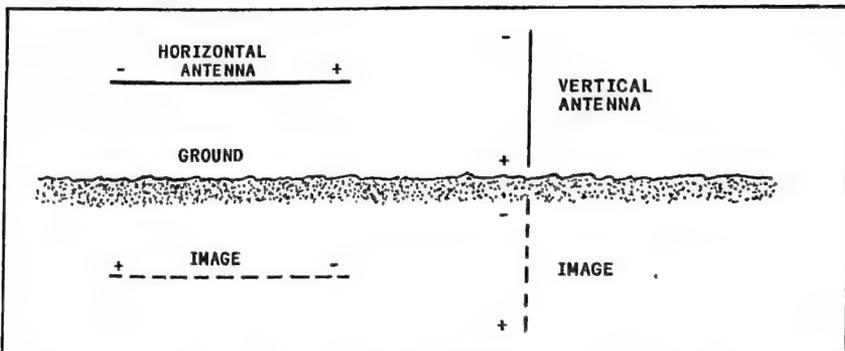
Fig 4-1 -- Horizontal and vertical antenna representations along with their in-ground image halves. Note the polarity change for the image portions.
