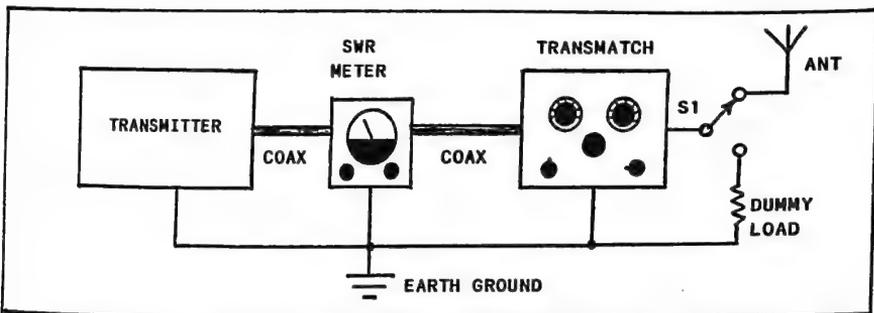
Fig 3-4 -- This is how your SWR meter is used when your Transmatch does not have a built-in SWR indicator. S1 may be included to permit switching from the antenna to a dummy load (see text). Coaxial cable should be used between units (50 ohms), between the Transmatch and the dummy load, and between the Transmatch and S1. The dummy load is used when making transmitter tuning adjustments. It is used also to obtain starting-point settings for the Transmatch.
