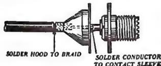
4) Slide hood over braid. Solder conductor to contact. Slide hood flush against receptacle and bolt both to chassis. Solder hood to braid as illustrated. Tape this junction if necessary. (For UG-177/U.)
