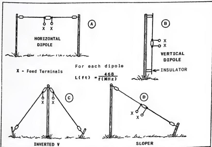
Fig 2-1 -- Examples of how half-wave dipoles may be erected. A figure-8 radiation pattern results from the arrangement at A. Antenna B has an omnidirectional pattern and vertical polarization. Antennas C and D also have vertical polarization and omnidirectional patterns assuming the enclosed angle at C is 90-100 degrees, and when antenna D slopes approximately 45 degrees toward ground from a nonconductive mast (see text).
