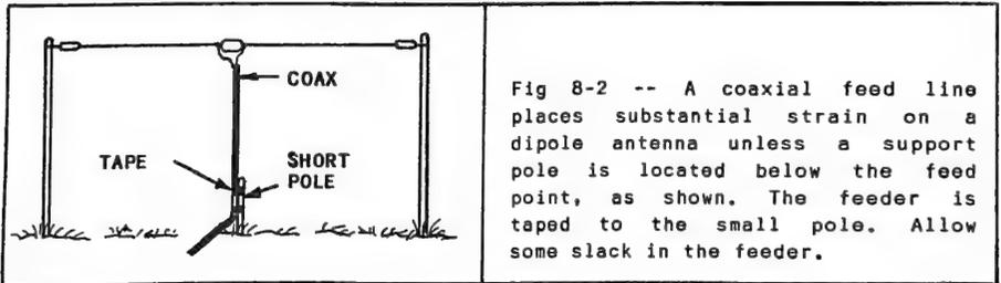
You may employ the method in Fig 8-2 for supporting open-wire or ladder-line feeders. These two feed lines are especially vulnerable to breakage at the antenna feed point when there is stress on the line. Two standoff insulators are required at the top of the short stabilizing post. The balanced feeder is attached to these insulators, rather than being taped to the post.
