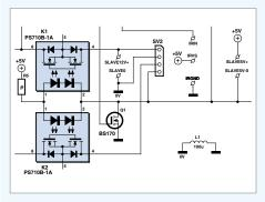
In Figure 2, the relay contacts are drawn incorrectly in their nonactuated state. which suggests all inputs are interconnected. Also, two miniature chokes are missing in the +12 V and -12 V supply lines. The corrected sections of the
