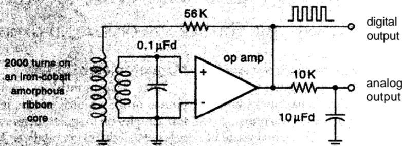
**FIG. 2-A RESONANT FLUXGATE MAGNETOMETER.** As before, the core will get switched in and out of saturation. The output duty cycle varies in proportion to the single axis field strength and direction. The high level output square wave is easy to interface to a PIC or other microcontroller.
