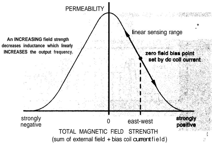
FIG. 3-SPECIAL ISOTROPIC MAGNETIC ALLOYS, whose permeability varies with field strength, are newly available. By biasing it as shown, a coil can be built so its inductance strongly varies with compass orientation.
