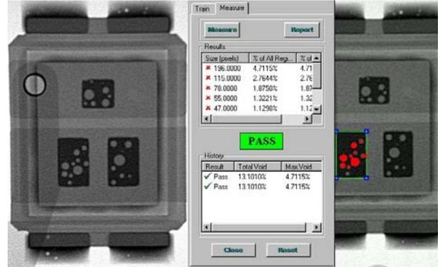
Figure 13 Voids on the left source contact
