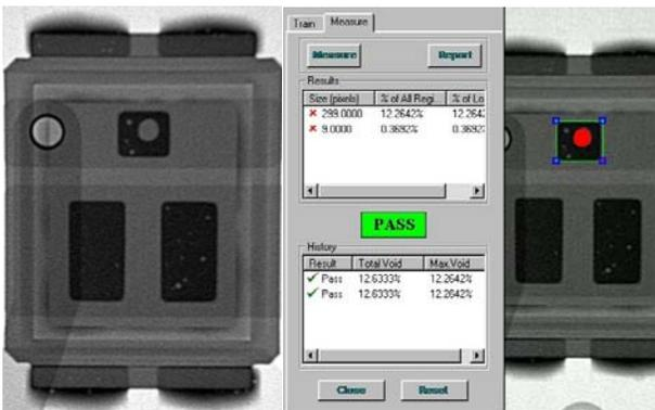
Figure 12 Voids on the gate contact
