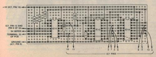
Above left is the revised memory address counter while at left is the suggested Veroboard layout which can be wired to the existing PC
