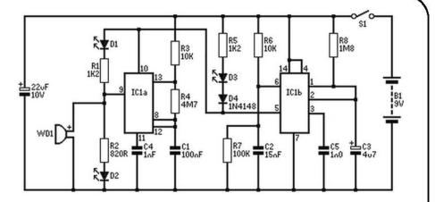
will only oscillate when the monostable output is high. The LED D1 must also be a source from this reset line so that it will go out when the monostable period is over. Consequently, the timer for the astable may have the supply
