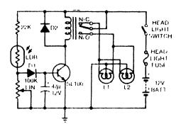
The circuit also operates without the power transistor 2N3055 (a saving). The LDR can be mounted on a small bracket screwed to the right head lamp's mounting screw after wrapping the LDR neatly in a single layer of polythene sheet.
