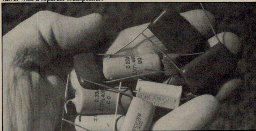
Old paper capacitors should be replaced with high voltage (400-630V) polyester equivalents.
