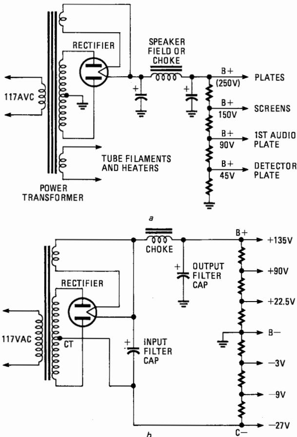
FIG. 4—BLEEDER DROPS THE B+ voltage for different stages of the receiver, while stabilizing the power-supply output (a); and (b) bleeder with negative end for bias.
