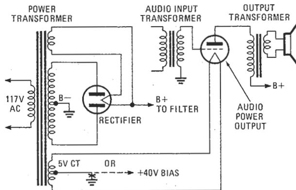
FIG. 1—FILAMENT CENTER TAP is the ground return for the "cathode" circuit. Bias may be applied at this point.
