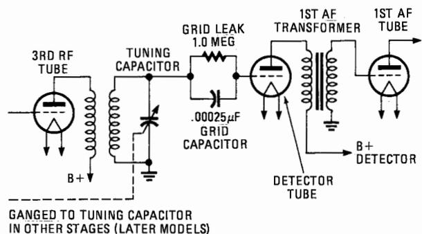
FIG. 5—GRID-LEAK DETECTOR USED in most old TRF radios. In many cases the "leak" resistor went direct from grid to ground.
