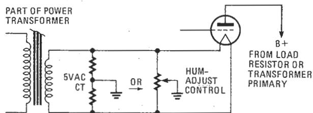
FIG. 2—LOW-OHM FIXED RESISTOR was often used instead of center tap. If adjustable, it could reduce hum. (Later ones on AC tubes were commonly called "humdingers.")
