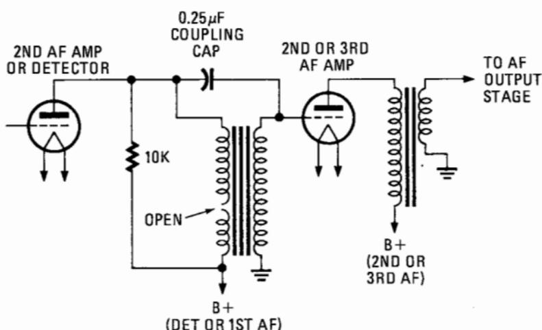
FIG. 6—"QUICK-AND-DIRTY" fix for an open AF transformer.
