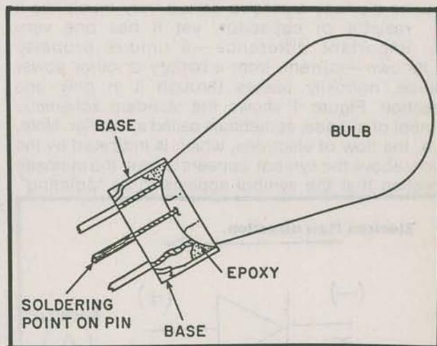
Mending a loose base is relatively easy, but involves more time and materials than cleaning. You will need some solder and a soldering iron, a hobby knife, epoxy, and desoldering braid. First, remove the old solder from the tube's pins with the braid (see illustration). After the pins are desoldered, gently remove the base, labeling each of the wires and the respective pins. This will be critical when the base is re-attached. Next, remove *most* of the old epoxy with
