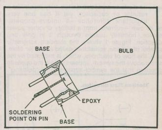
Mending a loose base is relatively easy, but involves more time and materials than cleaning. You will need some solder and a soldering iron, a hobby knife, epoxy, and desoldering braid. First, remove the old solder from the tube's pins with the braid (see illustration). After the pins are desoldered, gently remove the base, labeling each of the wires and the respective pins. This will be critical when the base is re-attached. Next, remove *most* of the old epoxy with
