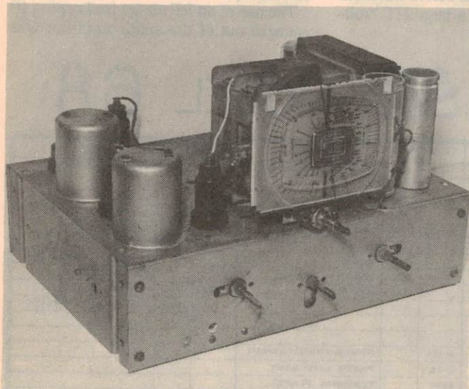
Fig.2 (left): The relatively small size of the metal valves and lack of shields gave the large chassis an uncluttered appearance. In a modern restoration the original wet electrolytic capacitors can be left for appearance, but should be disconnected and functionally replaced by modern components. Fig.3 (right): Component mounting boards and a roomy chassis make STC receivers ideal for the vintage radio novice to work on.
