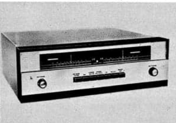
Harman-Kardon "Madrigal" ST350 stereophonic AM-FM tuner has push-button controls for Multiplex, AM noise filter, FM-AFC, FM, AM and stereo.
