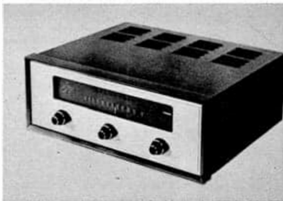
Fisher FM-100 tuner has main channel and Multiplex channel switch, four wide-band IF stages with limiters, bridge-connected mixer and oscillator.
