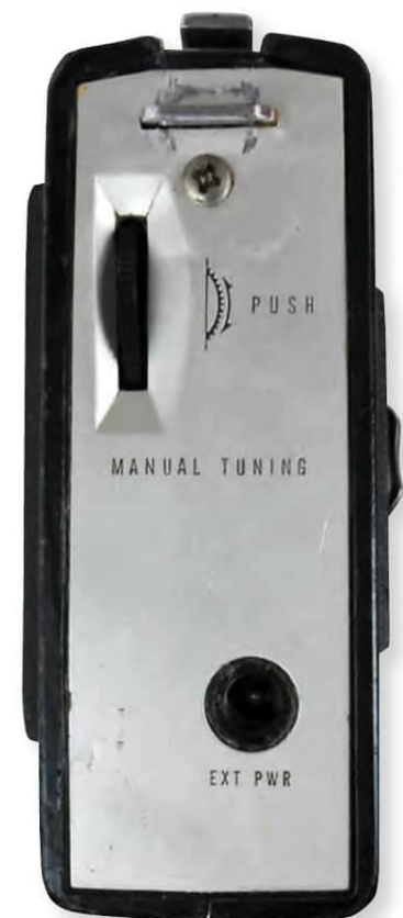
The left (above) and right (below) sides of the Radar Matic R-1000 shown at close to actual size. The case is plastic with a leather-like finish, while the grille and sides are metal.
