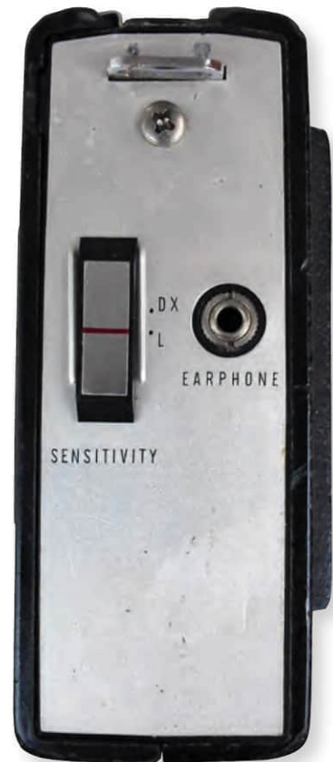
The left (above) and right (below) sides of the Radar Matic R-1000 shown at close to actual size. The case is plastic with a leather-like finish, while the grille and sides are metal.
