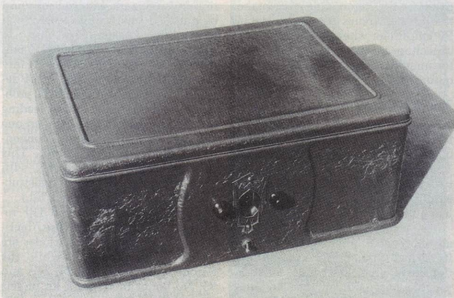
This 8-valve Apex receiver with its push-pull output stage performs rather well for an old TRF. Many budget-priced TRF receivers from the late 1920s were housed in pressed steel cabinets.
