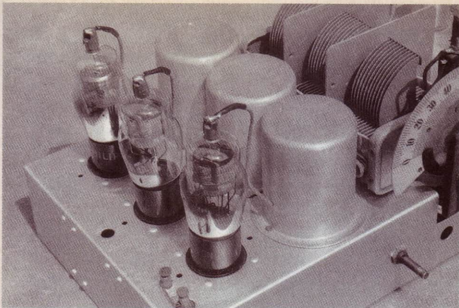
A typical layout for a TRF receiver – a tuning section with three valves, three coils and a three-gang tuning capacitor, all neatly arranged side by side. In addition, this receiver employs an output valve and a rectifier valve, giving five valves in total.
