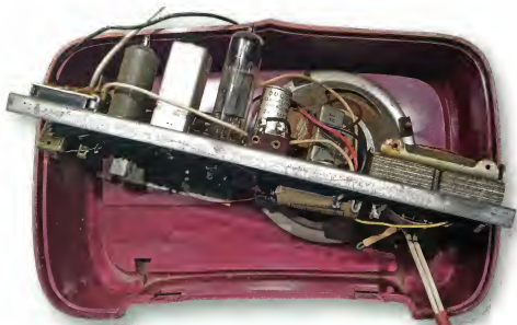
The DLP's chassis sits at an angle inside the cabinet so that it fits in the allotted space. This view shows the set prior to restoration. The 2-core mains flex was later replaced with 3-core mains cable so that the chassis could be earthed.
