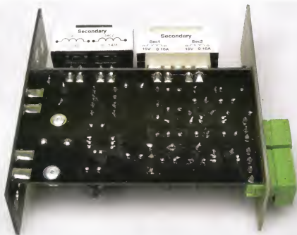
The underside of the PCB assembly showing how the main board, transformer board and front panel are soldered to each other. The rear panel (right) is not secured at all but is held loosely in place by the two output sockets. The main board is soldered 2mm down from the edges of the transformer board and panel.
