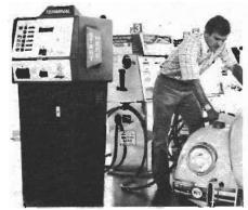
Automated service station in Anaheim provides for fast, efficient self service. A customer simply inserts his credit card (or cash) in a control panel on the pump island, presses a button to select his fuel, proceeds to the designated pump and pumps his own gas. A detailed receipt is issued once the transaction is complete.
