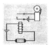
After tuning the Coherer, connect it up to a circuit like that shown at right, below. The circuit can be provided with a de-
