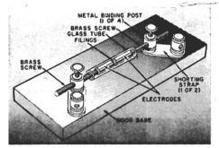
Parts must be solidly mounted on the wood base. Screw-type metal binding posts will facilitate easy mounting of the electrode assembly and will also provide convenient circuit connections.
