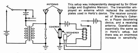
ed of Branley's Coherer, a Popov decohering device, and a receiving antenna. Operation was essentially the same as in Hertz's setup, but there was an enormous increase in sensitivity.
