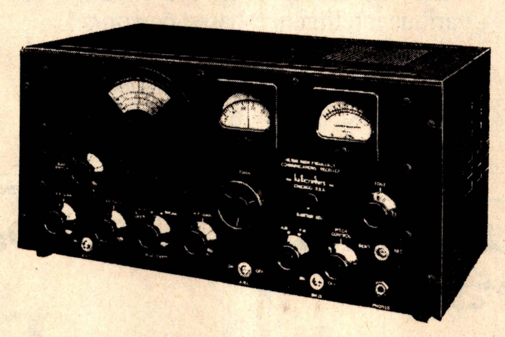
Hallicrafters Made Fig.5: Incorporated of Chicago, the S-27 receiver had 15 valves and tuned from 27MHz to 145MHz in three ranges. It also demodulated FM, and allowed the British to finally detect the German Knickebein beams.
