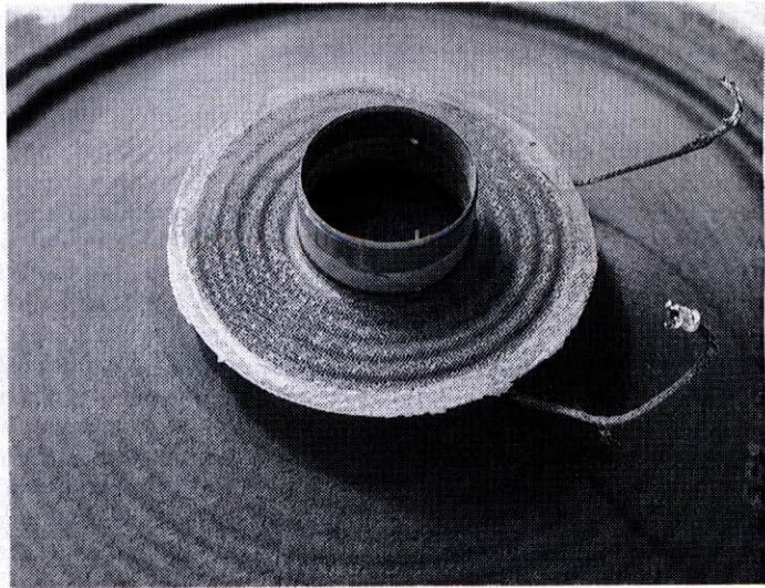
Fig.5: Inexpensively moulded from varnished or plasticised cloth, the modern spider is non adjustable. Simply glued to the chassis, it doubles as a dust seal for the voice coil.
