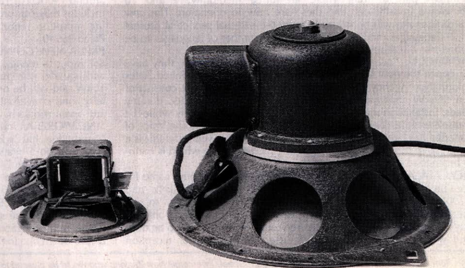
Fig.2: Moving coil loudspeakers are remarkable for their diversity of sizes, and this pair are by no means extremes. At the left is a 5" AWA unit made around 1935. The other is a 1930 Atwater Kent type N, about 11" in diameter.
