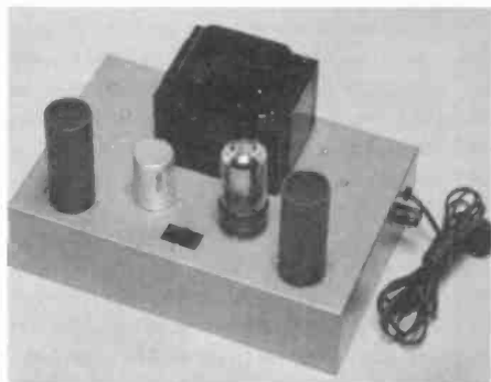
Fig. 8. Top view of power supply chassis.
