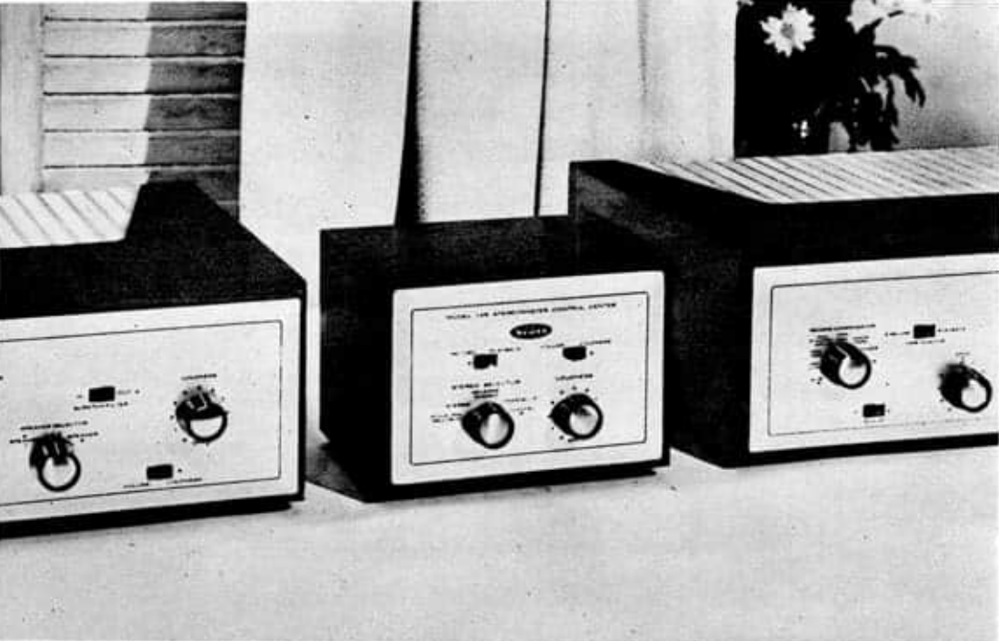
H. H. Scott stereo adaptor sells for $24.95, is used to convert two separate monaural systems to stereo. The drawing below, right, shows how this unit controls and mixes both channels of a stereo program.
