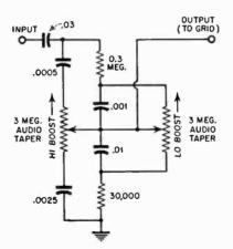
The network is shown at left and the values shown give substantially the same response curves as shown in the article. The input should be connected to a source impedance not higher than about 20,000 ohms, to prevent loss at high frequencies when in the high boost position, and the output should work directly into a grid, as pointed out in the editorial note.
