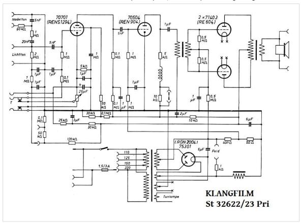
The Klangfilm St-32 622, RE604 PP, 1928-32 are partly made with the same current loop bias as the SE versions. The first stage RENS1294, listed as a HF *exponential* pentode (Whatever that means) has the auto cathode bias that we are familiar with. The second stage is a nice interstage triode phase splitter – again – however – with that degrading resistor in series. (Is it there to protect the primary winding in case of tube failure?)
