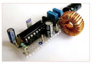
series, the 4xxx series isn't as picky as regards supply voltage, happily working at supply voltages ranging from 3 to 18 V. And this application doesn't require the buffers to switch rapidly anyway. Of the six available buffers in IC1 (a 4050), two are placed in series to furnish adequate levels of amplification. The remaining four buffers are connected in parallel to the second buffer, which improves the way the transistors are driven.
