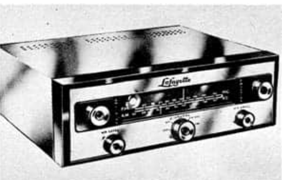
Stereo tuner kit by Lafayette costs $74.50, has Armstrong FM circuit with 5 Kc maximum drift. It comes with prealigned IF's, plus printed circuits.
