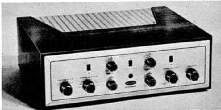
Type 229 stereo dual 20-watt amplifier and preamplifier is rated at 17 watt of continuous power for each channel, has a phase reverse and stereo balance control. Outputs include tape and 4, 8 and 16 ohm.
