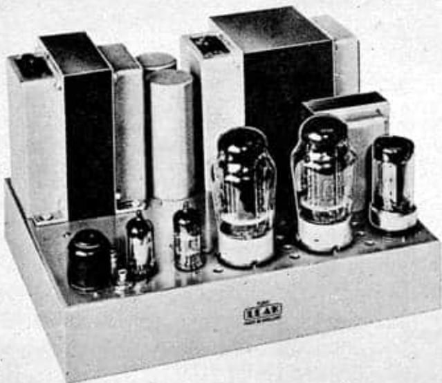
Leak, British 50-watt monaural amp can be used with speakers having impedance of 3 to 20 ohms. Response is 20-20,000 cps  $\pm$  .5 db; price is \$149.
