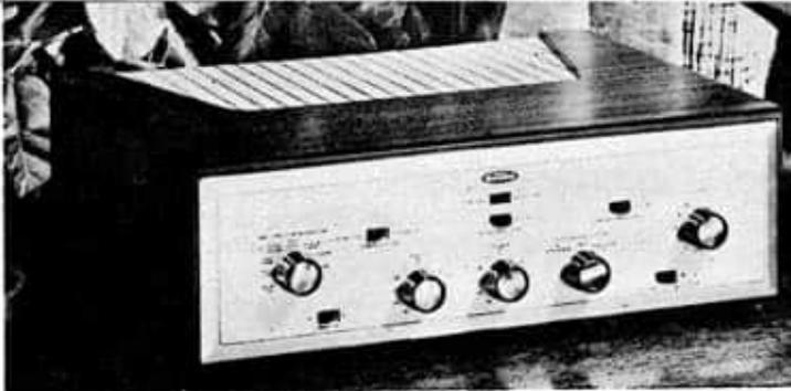
Dual 12-watt amplifier and stereo preamp, Model 222, has noise and hum of 80 db below full power output; harmonic distortion is .8%. It has a third channel amplifier jack.
