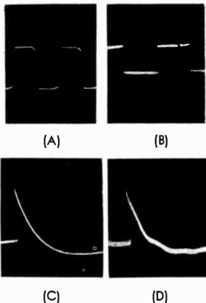
Fig. 6. Oscillograms of output for various input signals: (A) 200-cps square wave; (B) 5000-cps square wave; (C) 0.5-volt d-c pulse at input, speaker connected normally; (D) same signal as at (C), but with 10-ohm resistor in series with voice coil. Last two oscillograms show effect of damping.
