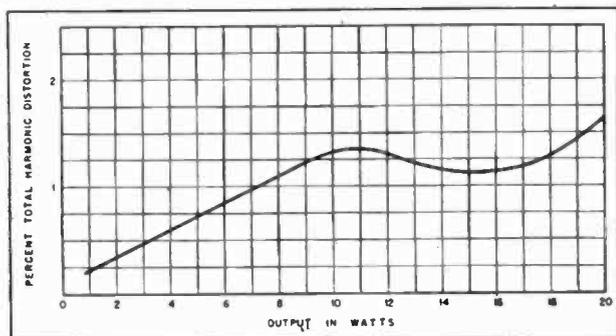
Fig. 5. Total harmonic distortion vs output at 50 cps.
