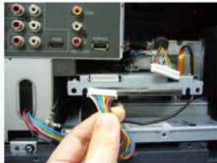
2. Disconnect the Wire from Power BD
