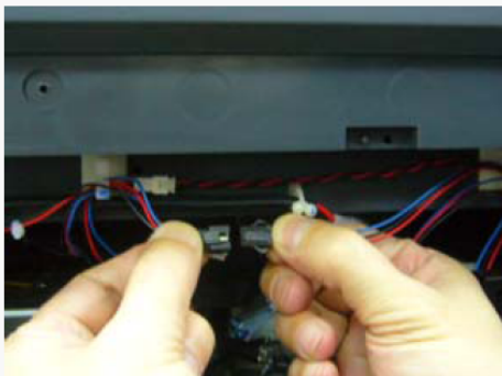
2. Disconnect the Optical Fan Wire
