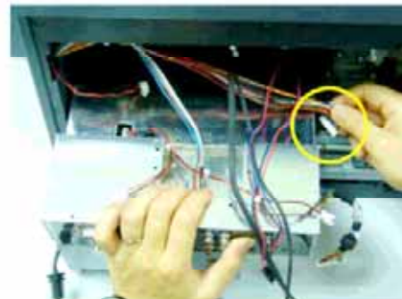
2. Disconnect the Function Key Wire
