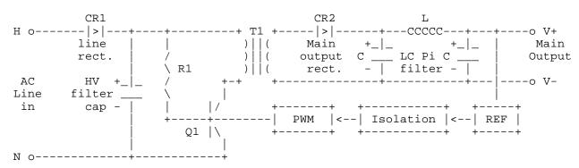
Probably the most common topology for small switchers is the flyback circuit shown below:
