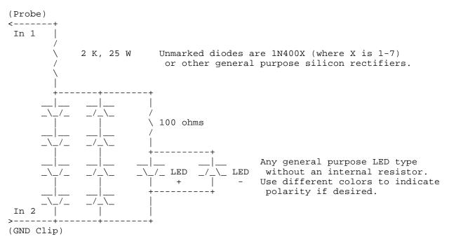
The two sets of 4 diodes will maintain a nearly constant voltage drop of about 2.8-3 V across the LED+resistor as long as the input is greater than around 20 V. Note: this means that the brightness of the LED is NOT an indication of the value of the voltage on the capacitor until it drops below about 20 volts. The brightness will then decrease until it cuts off totally at around 3 volts.
