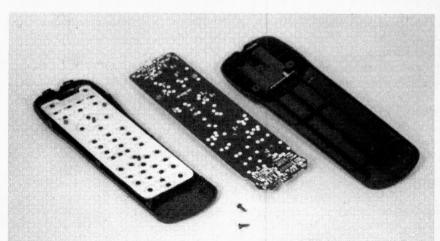
REGARDLESS OF THE CAUSE OF THE PROBLEM, servicing a remote means getting inside. If the means of fastening the two case halves is not obvious, look for screws inside the battery compartment or under a label on the rear.
