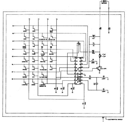
INSIDE A TYPICAL TV/VCR remote control transmitter. This schematic is for a unit made by Zenith.
