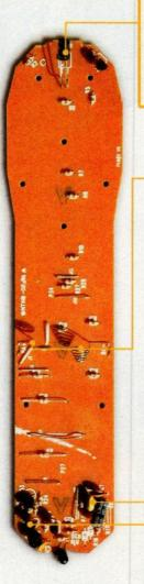
backlighting for the buttons. The infrared LED and the transistor to drive the current for the LED provide the interface to the outside world to control
