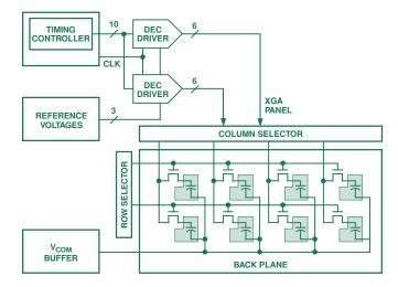
Figure 1. Simplified view of an XGA microdisplay panel driven by two DecDriver ICs.
