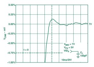
Figure 6. Typical DecDriver output settling time.
