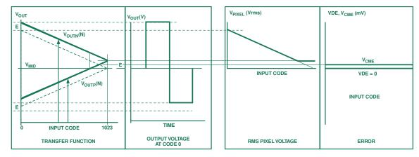
Figure 4. A typical example of  $V_{CME}$  or common-mode (offset) error. As in Figure 3, AD8380 transfer function, time-domain rms signal at code zero, rms voltage seen by the pixel, and the  $V_{CME}$  error as a function of DAC code.
