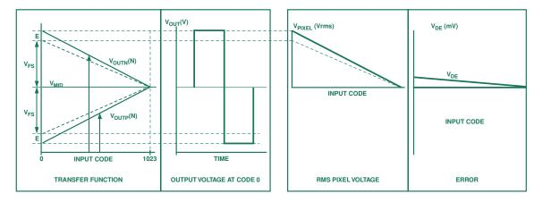
Figure 3. A typical case of  $V_{DE}$  or differential error. From left to right, plots show transfer function, time-domain rms signal at code zero, rms voltage as seen by the pixel, and the error vs. DAC code.
