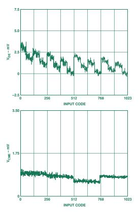
Figure 5. Typical  $V_{\text{DE}}$  and  $V_{\text{CME}}$  as functions of input code.
