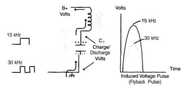
Fig. 2: The intensity of the flyback or coil's magnetic field determines the charging current to Cr and amplitude of the induced voltage pulse.
