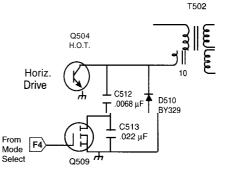
Fig. 6: Capacitor switching in series changes the timing of the output stage for proper high voltage and/or deflection at a different frequency.
