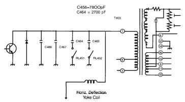
Fig. 5: Switching capacitors in parallel increase the C+ total value to reduce the flybackpulse amplitude at low frequency modes.
