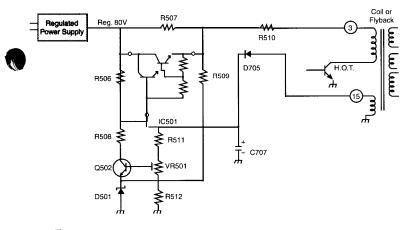
Fig. 7: Example of a linear high voltage/deflection B+ regulator in a multi-mode computer display monitor.
