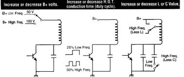
Fig. 3: Methods of altering the horizontal output stage to keep the high voltage and deflection constant at new operating frequencies or modes.
