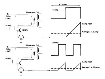
Fig. 1: Increasing the horizontal frequency reduces the average flyback or coil current and input energy to the horizontal output stage.
