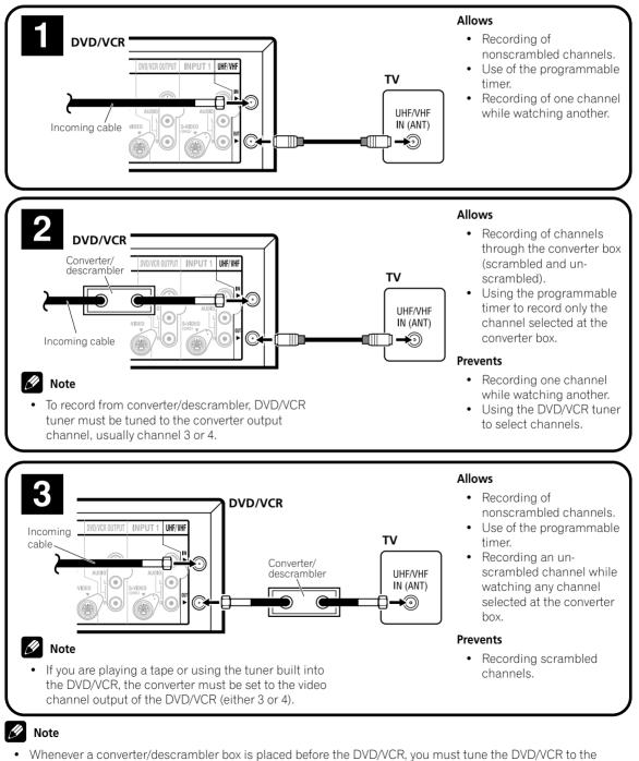
Whenever a converter/descrambler box is placed before the DVE output of the converter/descrambler box, usually channel 3 or 4.
