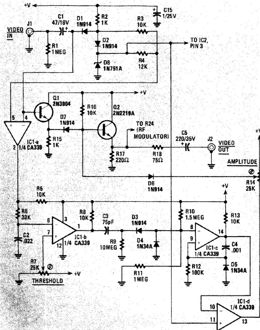
FIG. 3—DETECTION AND REGENERATION of vertical-sync pulse are performed by IC1.
