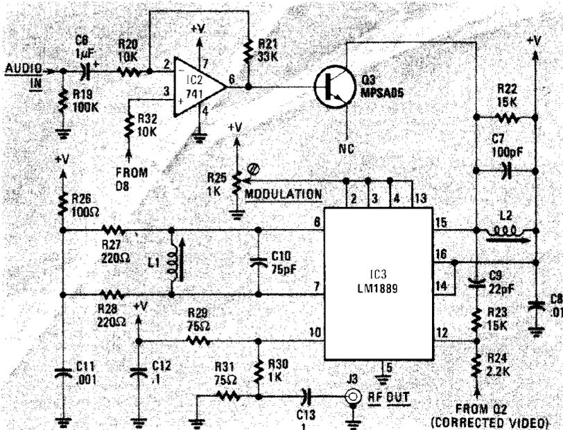
FIG. 4—RF MODULATOR. Capacitor C13 at RF OUT jack may be replaced by vestigial-sideband filter if desired (see text).
