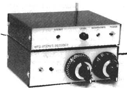
AN OUTBOARD TUNER lets you use the circuit with a TV that lacks audio outputs. Next time, we'll see many other ways of using the circuit.
