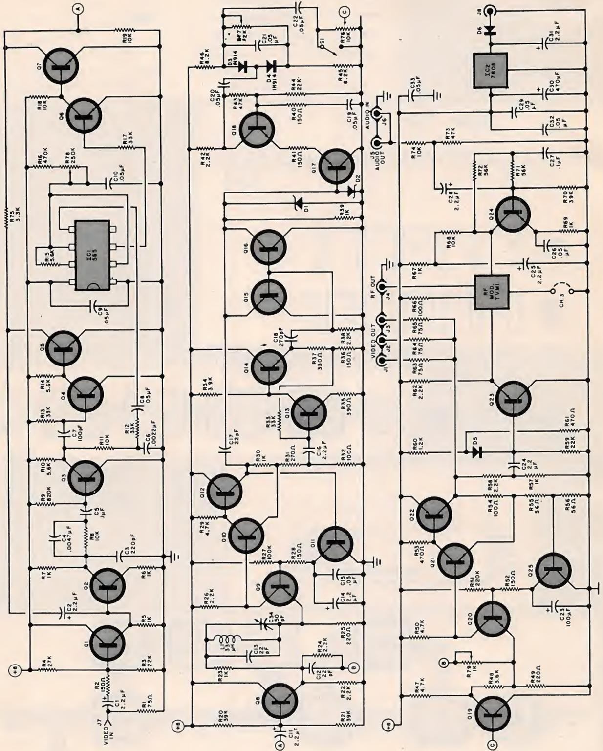
Fig. 6. Schematic diagram of Video Enhancer.
