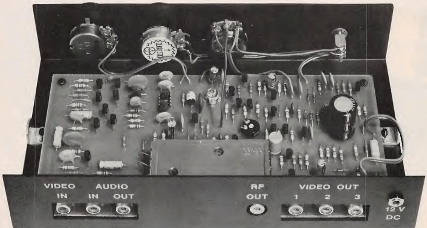
Photo shows interior construction details of the Video Enhancer.
