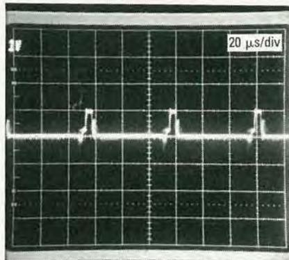
FIG. 24—THERE IS NO VIDEO at IC2 pin 3.
