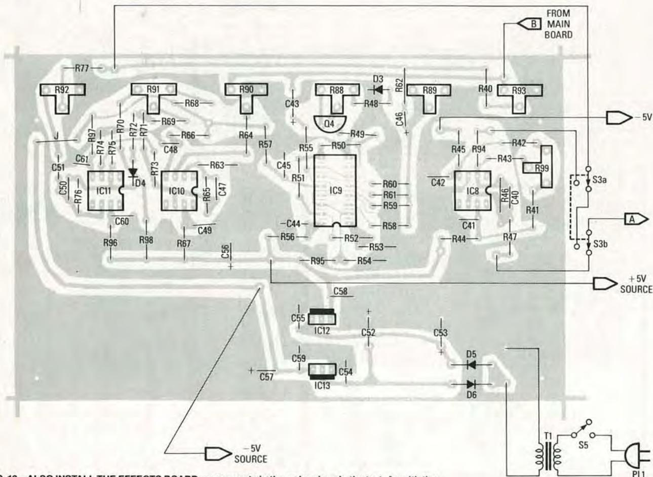
FIG. 13—ALSO INSTALL THE EFFECTS BOARD components in the order given in the text. As with the main board, IC sockets are suggested to simply troubleshooting.
