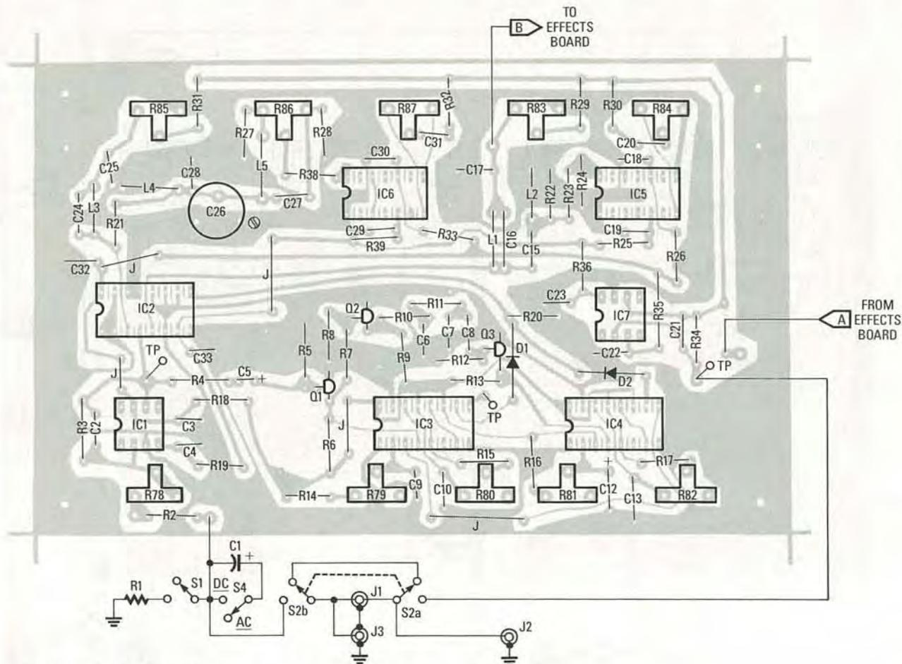
FIG. 12—INSTALL THE MAIN BOARD COMPONENTS in the order given in the text. While IC sockets aren't specified, their use is suggested. They make troubleshooting easier if you have any problems.
