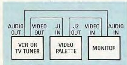
FIG. 14—USE THIS KIND OF HOOKUP for checking and aligning the video palette. A TV-tuner signal source can originate in the VCR, or use an integral TV-tuner device.
