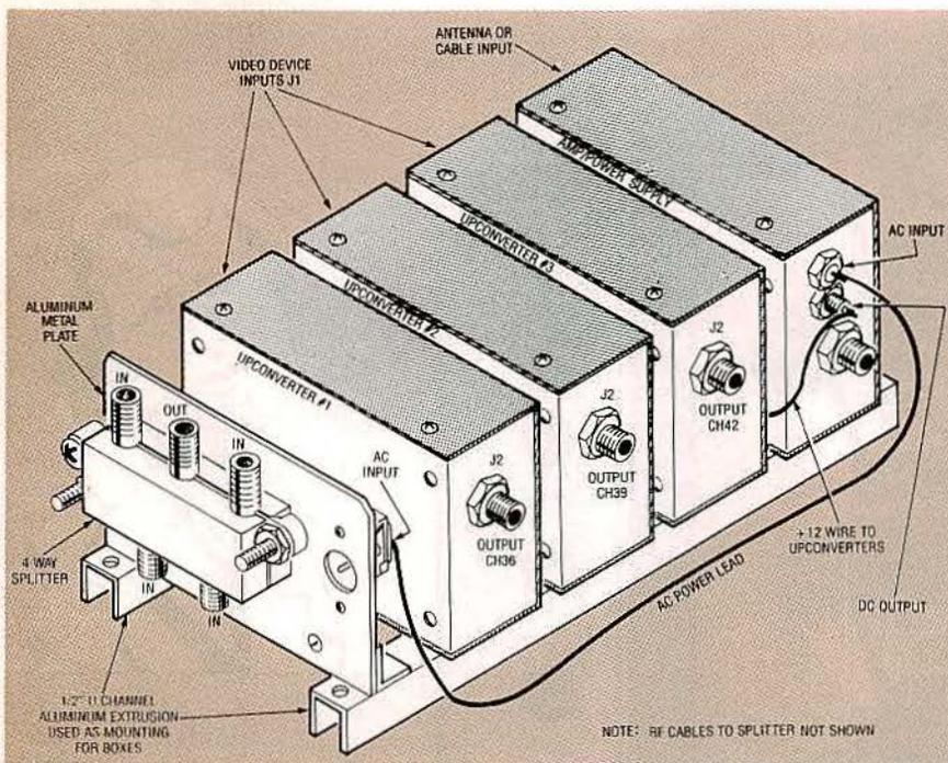
FIG. 11—ALL OF THE MODULES for the prototype Video Master are mounted together on a pair of aluminum rails, with everything feeding into a 4-way splitter mounted on one end of the assembly.
