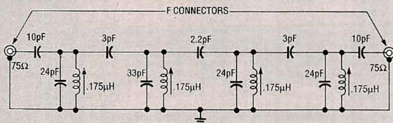
NOTE: FILTER IS SYMMETRICAL — INPUT AND OUTPUT ARE INTERCHANGEABLE
